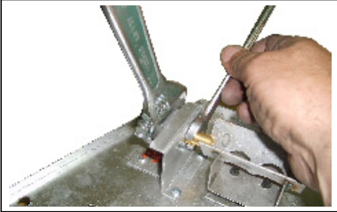
Figure 83 - Use two wrenches to avoid damage to manifold.
