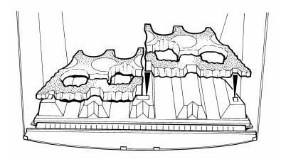
c) Place the Front Ceramic Rails centrally onto the Semi-Circular location plate situated at the front of the burner. Ensure that the front ceramic rails are located over the front edge. (See below)
