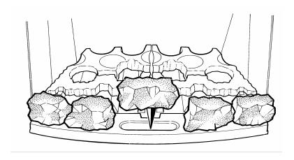
e) Select four of the large coals and two small coals, and place them on the front of the fuel bed directly behind the spaces between the front row of coals.
