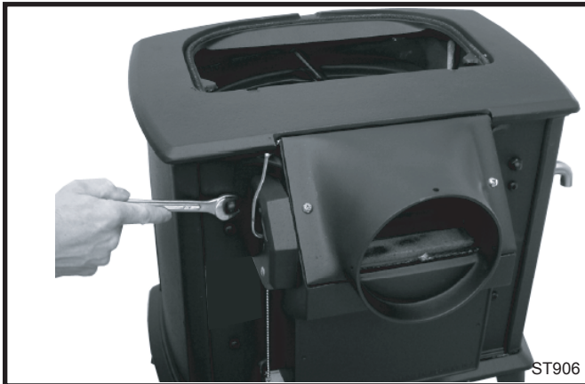
Fig. 37 Loosen damper assembly bolts.
