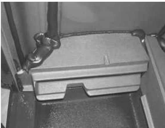
Fig. A-7 Cement on left air tube for left air wash manifold
