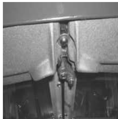
Fig. A-8 Center bolt on air wash manifolds
