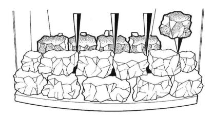
g) Place the remaining four large coals as shown below (Taking care not to allow the coals to be trapped behind the fuelbed):-
