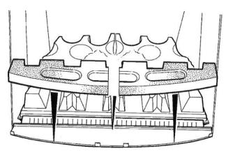
d) Select five of the large coals and locate each one centrally into the depressions in the Front Ceramic Rail. Ensure that the coals are equally spaced as shown below.
