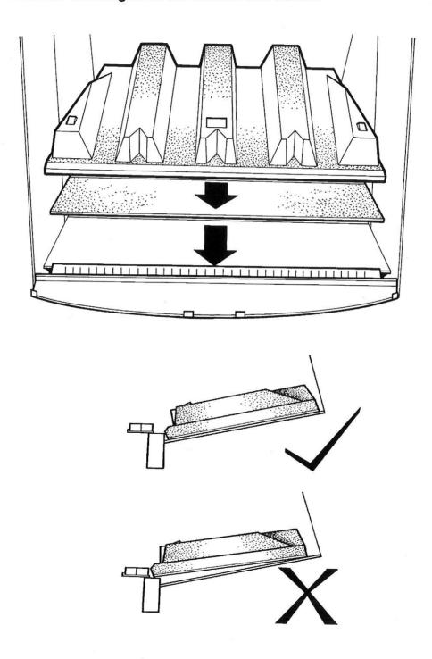
b) Place both the hard ceramic fuel bed sections on to the base so that the location lugs fit snugly into the recesses on the fuel bed sections.
