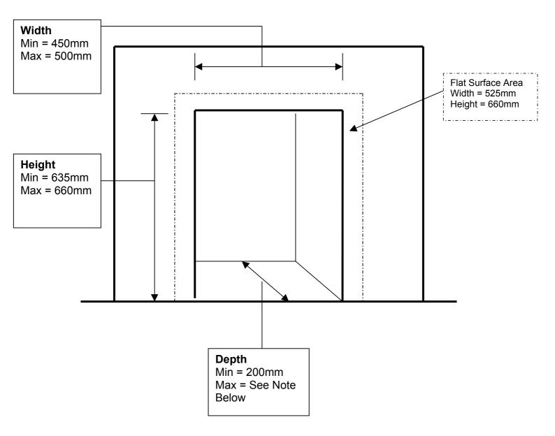
**NOTE** : Maximum dimensions when measured on individual installations must not calculate to exceed a void volume of  $247 \text{dm}^3$ , or be less than  $12 \text{ dm}^3$ . See page 14 for example calculation.
