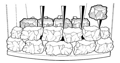
g) Place the remaining four large coals as shown below (Taking care not to allow the coals to be trapped behind the fuelbed):-
