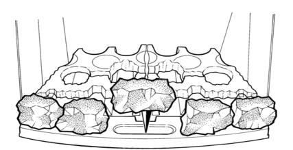
e) Select four of the large coals and two small coals, and place them on the front of the fuel bed directly behind the spaces between the front row of coals.
