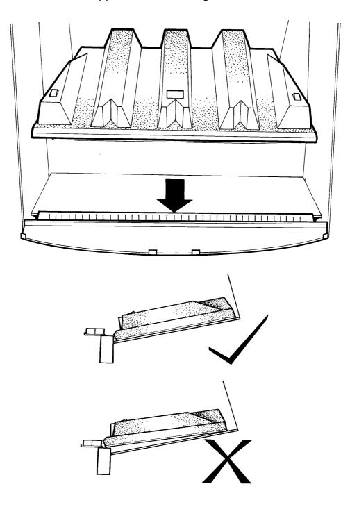
b) Place both the hard ceramic fuel bed sections on to the base so that the location lugs fit snugly into the recesses on the fuel bed sections.
