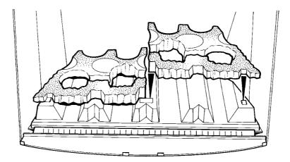
c) Place the Front Ceramic Rails centrally onto the Semi-Circular location plate situated at the front of the burner. Ensure that the front ceramic rails are located over the front edge. (see below)
