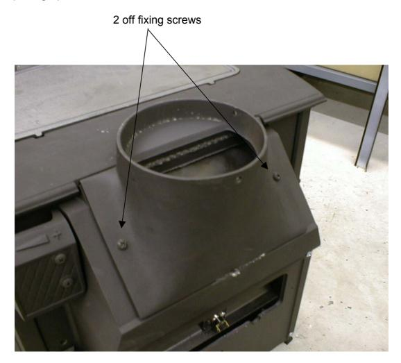
b) Take care to lift the flue spigot collar away from the stove. Rotate the flue spigot collar through 180 degrees clockwise, taking care not to damage the rope seal. Ensure that the rope seal is correctly positioned, when refitting to the appliance. (see photograph overpage).
