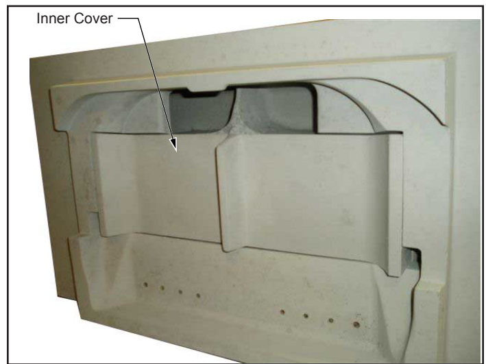
Figure 3.11 - Remove inner cover.
