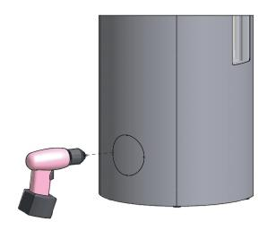
Drill out the four holes in the cover plate with a  $\phi 8$  bit and remove the plate.
