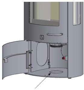
The cover plate at the bottom of the wood-burning stove is removed and outside air is connected to the connection piece underneath the combustion chamber.
