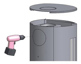
Undo and remove the blanking plate from the inside.
