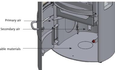
For security reasons it is not allowed to store flammable materials under the combustion chamber of the Scan 59.
