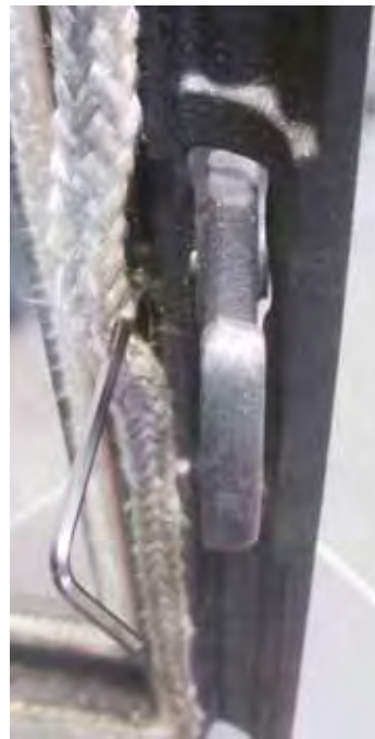
Grub screw hidden by the door rope seal on some models
