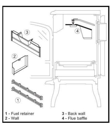
First remove the log retailing guard (1) which is made up of two identical parts (FB307422).
