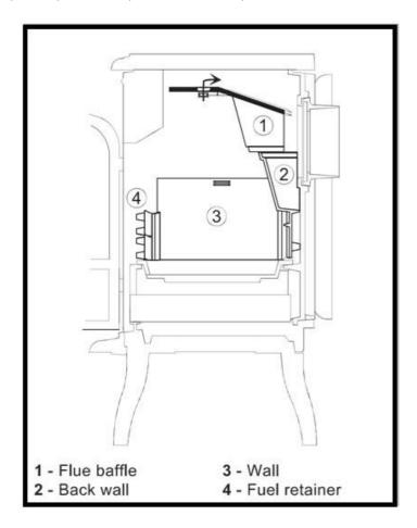
Angle the baffle to get it through the door and then lift it So that the cut outs on the baffle allow the baffle to be lifted so that it can be slid backwards supported by the castings on the side walls of the stove.
