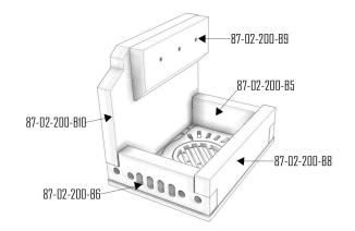
Left side brick b10 and then fix the additional side brick B9 to it using the three stainless screws.
