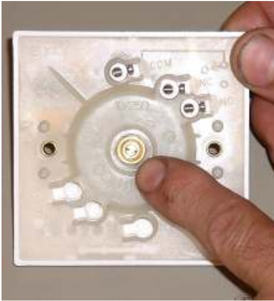
3.4 Fig 2 Time delay adjusting screw
