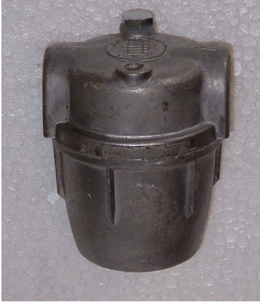
FIRE VALVE. FIG 4 Check for function and leaks.
