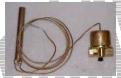
When fitting the fire valve make sure that where the capillary and oil line go through the bulkhead in separate sleeved tubes, so that the capillary can be withdrawn separately should it ever need replacing.
