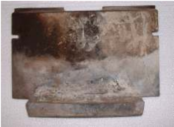
Fig 12. Secondary air chamber casting removed.
