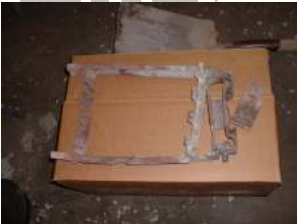
FIG 9. REMOVE THE RIDDLING GRATE SUPPORT FRAME.
