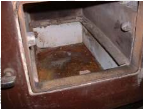
Fig 13. Remove the ash pit base plate casting.
