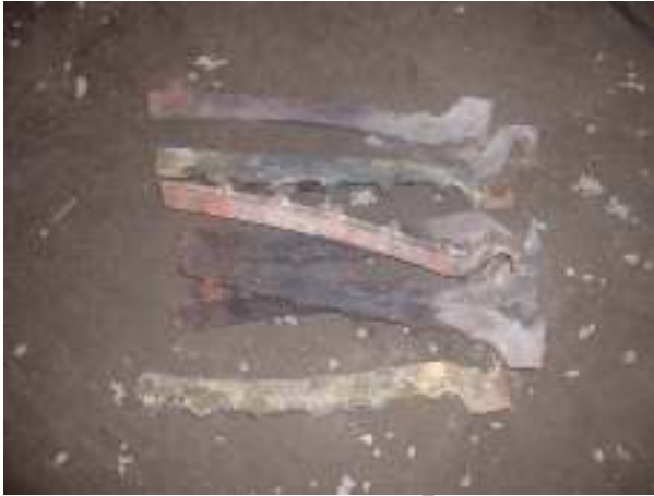
Fig 8. Remove the grate bars by lifting them up from the back support.
