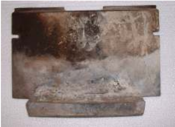
Fig 12. Secondary air chamber casting removed.
