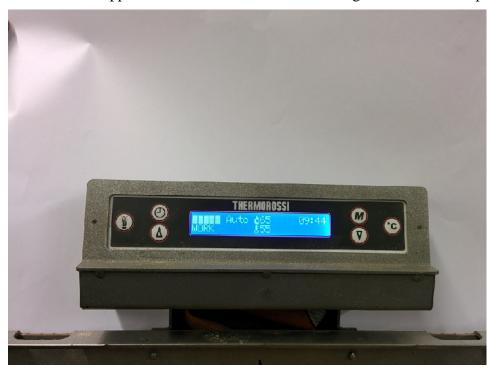
2-3. To get the controler into the 'adjust parameters' display; hold down the two arrow buttons on the panel at the same time for TEN SECONDS as illustrated below.
