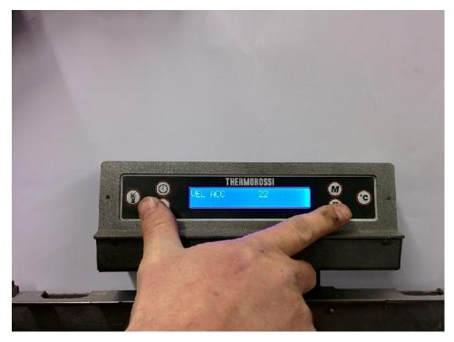
2.4. After the up – down arrows have been depressed for ten seconds, the first parameter "VEL ACC" will appear, the VEL ACC parameter should be 22.
