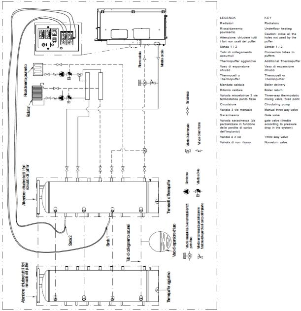
CAUTION: The system operating pressure must always be above the expansion tank preload: 2 bar for the expansion tank 1,5 bar.
