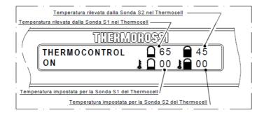
The figures relating to the Sensor S1 setting begin to blink. Press button (4) and/or (3) to set the action temperature for Sensor S1.
