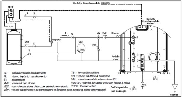
In order to guarantee correct absorption of the heat produced by the generator is it is advisable to use a boiler tube with volume and heat exchange capacity suitable for the power of the generator.
