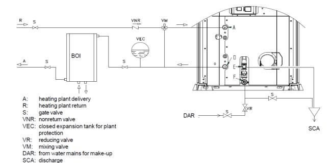
CAUTION: The water temperature in the boiler tubes in this case is not adjustable and depends on the systems's delivery temperature, that is the max temperature t setting.
