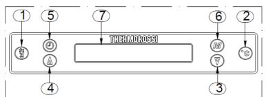
To set the clock and the day of the week carry out the procedures described below. Press button (6) repeatedly until the word **DATE** appears on the Display (7); wait a few seconds for the following indications to appear on the Display (7):
