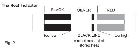
The heat indicator is above the Roasting Oven door and has three sections: black, silver and red. When the indicator is on or around the black line in the silver section the cooker is at the correct working temperature. The purpose of the heat indicator is to show whether the cooker contains the full amount of stored heat and it should be, therefore, only be referred to first thing in the morning or after a period of several hours during which no cooking has been done.
