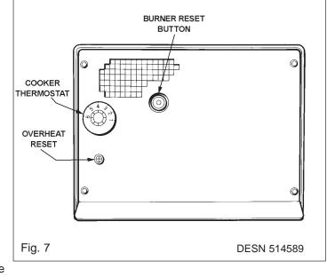
Continued lockouts indicate a burner or oil supply fault. This should be investigated and rectified.
