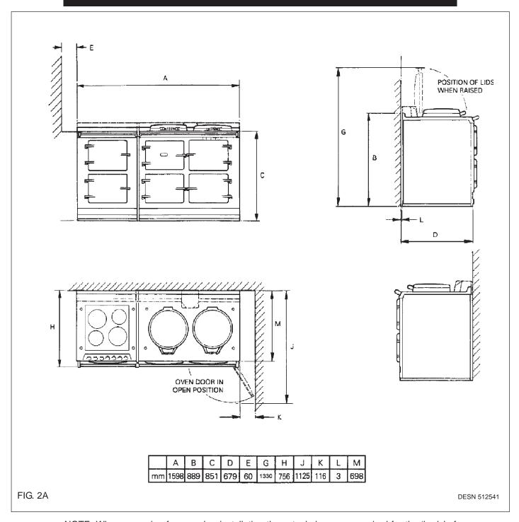
NOTE: When surveying for a cooker installation the actual clearance required for the 'body' of the appliance should be increased overall by 10mm beyond the figures quote above. This allows safe margin to take into account the natural dimensional variations found in major castings in particular the width across an appliance recess could be critical.
