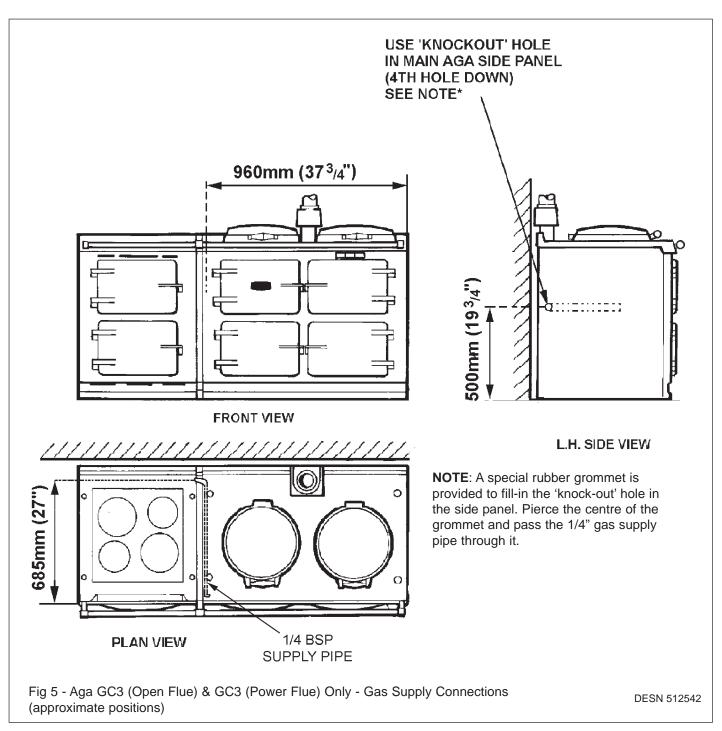
**NOTE**: For gas supply to the Aga GC3 use <u>EITHER</u> the supply pipe as shown above, <u>OR</u> the supply pipe (also provided) with gas inlet low down at front right hand side of Aga GC3. (see Fig. 1 of GC3 Installation Instructions).
