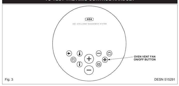
Press the fan button on the handset, the vent fan symbol should show on the handset screen.
