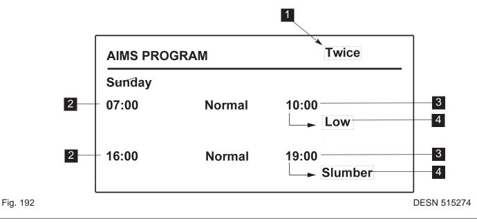
This screen shows that the ovens will be up at 'Normal' temperature between 07:00 and 10:00, the ovens will then go to 'Low' mode.
