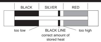
The heat indicator is above the Roasting Oven door and has three sections: black, silver and red. When the indicator is on or about the black line in the silver section the cooker is at the correct working temperature. The purpose of the heat indicator is to show whether or not the cooker contains the full amount of stored heat when the cooker is in its normal operational mode. During cooking the indicator line will drop back. This is normal and the heat will be automatically restored.
