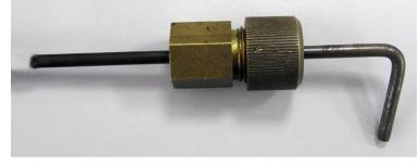
To remove the assembly from the burner inlet pipe. Hold the tube with mole grips or an adjustable spanner at the "T" connection where the oil feed from the valve joins the pipe. Then using a 22mm spanner undo the big brass nut from the inlet pipe. If the knurled nut has seized in place, soak the assembly in a penetrating oil or clean heating oil until it can be unwound.
