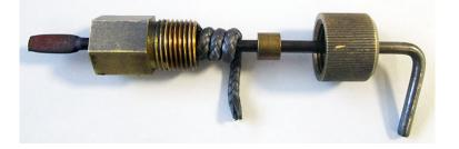
Slide the brass bush down onto the rope and then tighten the knurled nut down onto the main body until the gland holds the rod tight.
