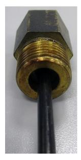
You will then require a small flat bladed screwdriver to dig out the old rope seal gland. It may be possible to pull out the rod from the body of the assembly prior to removing the gland but sometimes the gland has to be removed first.
