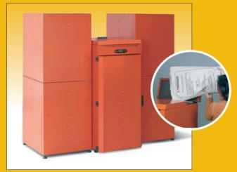
In addition to a built-in pellet storage capacity of 65 kilos, model COMPACT 18 and 32 can have one or two, optional, extra pellet storage hoppers of 100kg capacity each, fitted on the right, left, or both sides of the boiler, increasing the fuel capacity up to a maximum of 265 kilos.
