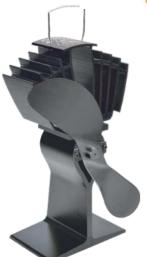
The Caframo AirMax Ecofan 812 is a heat-powered fan designed to circulate the warm air created by a wood-stove operating with normal surface temperatures of between 85°C and 345°C. The AirMax Ecofan 812 generates up to 175 Cubic Feet (of Air) per Minute. (At 85°C the AirMax Ecofan 812 will move 50 CFM)
