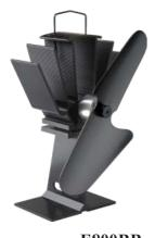
The Caframo Original Ecofan 800 is a heat-powered fan designed to circulate the warm air created by a wood-stove operating with normal surface temperatures of between 110°C and 345°C. The Original Ecofan 800 generates up to 100 Cubic Feet (of Air) per Minute. (At 110°C the Original Ecofan 800 will move 50 CFM)
