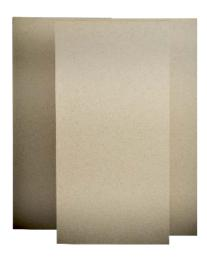
Board made from Exfoliated Vermiculite and has a high temperature resistance suitable for hotface applications up to 1100°C. The boards are easily cut to size with woodworking tools, the linings contain no ceramic or Asbestos fibres are non-dusting, non-irritant and odourless.
